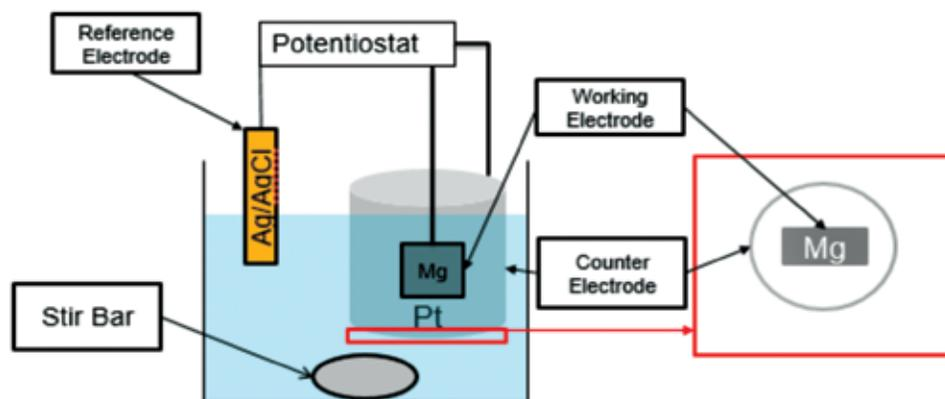
**Figure 1: Schematic of the electrode placement for the anodization procedure.** Electrolyte solution consists of 10 M KOH. A) Schematic of the anodization circuit. B) Schematic of Mg and Pt electrode configuration from a bottom-facing view.
