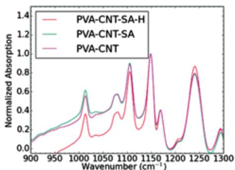
**Figure 6:** FTIR data for carbon nanotubes membranes.
