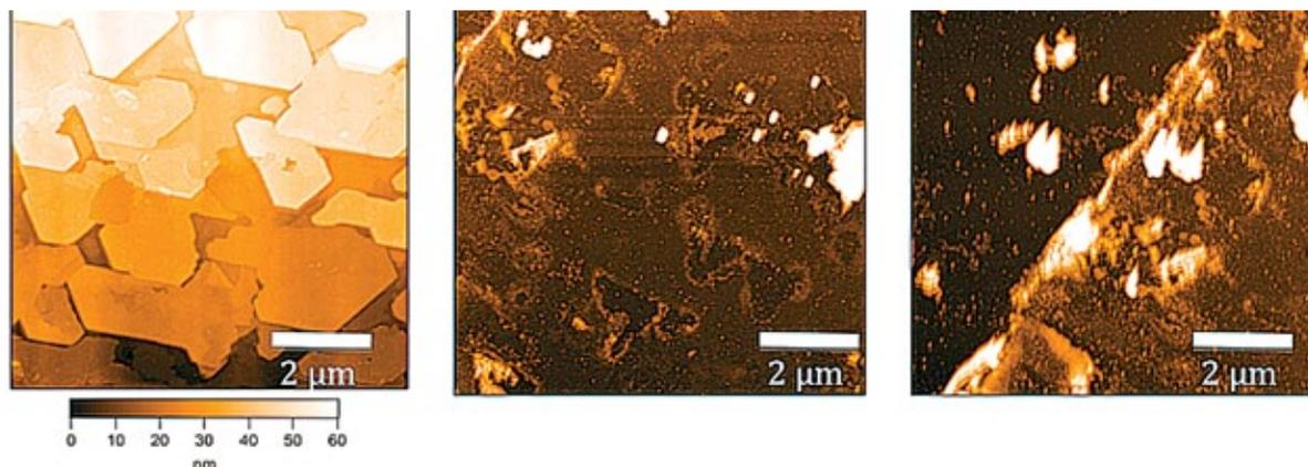
**Figure 6:** AFM images on the same scale of GeH before and after transfer. (a) 2.5 nm GeH on Ge(111). (b) 1.5 nm GeH continuous film after transfer. (c) 1.5 nm GeH step to underlying Si/SiO<sub>2</sub> substrate.
