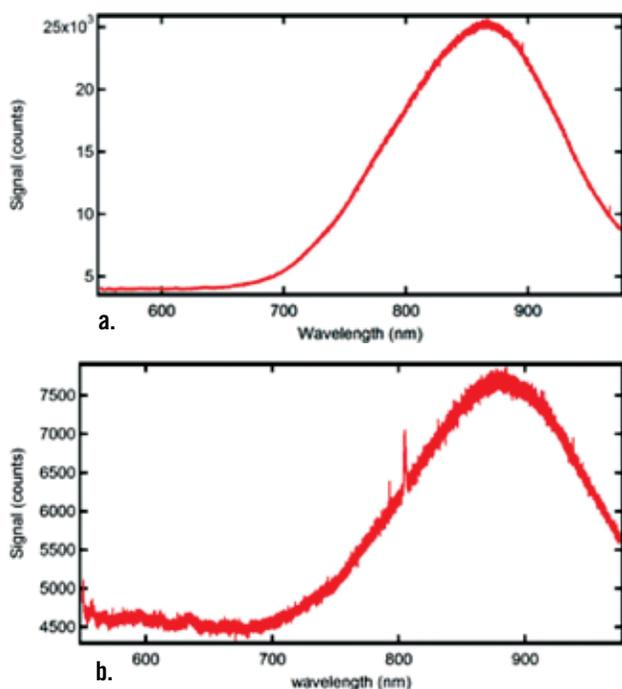
**Figure 7:** Photoluminescence spectra of germanane films on Ge(111) at 77K. (a) Pre-transfer. (b) Post-transfer.
