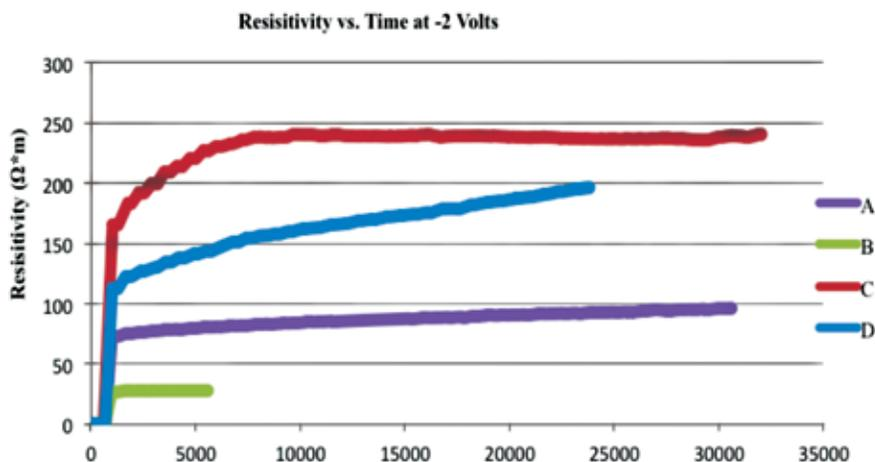
**Figure 7:** Graph of resistivity change of membrane during experimentation with electrical potential difference of -2 volts. (Membrane A: Heated for 4 hours at 80°C; Membrane B: Heated for 2 hours at 80°C and 2 more hours at 120°C; Membrane C: CNT solution was pretreated and heated at 80°C for 2 hours and the membrane was heated for 2 hours at 120°C; Membrane D: Heated for 4 hours at 80°C)
