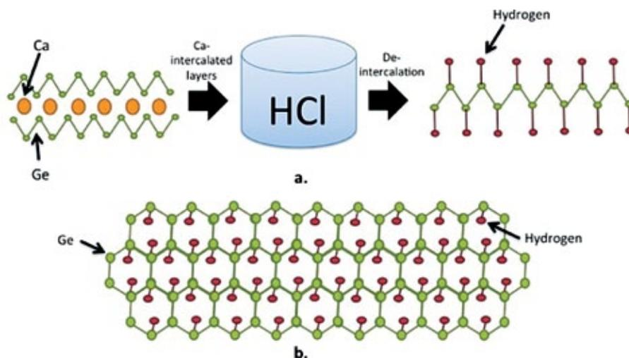
**Figure 1: Synthesis of Germanane.** (a)  $\text{CaGe}_2$  de-intercalation in  $\text{HCl}$ . (b) Monolayer  $\text{Ge}$  stabilized by hydrogen.
