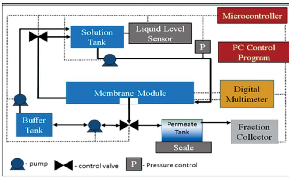
**Figure 4:** Schematic of the membrane testing process.
