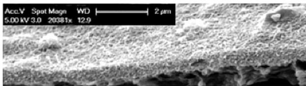
**Figure 3:** Cross section view of a membrane with PVA and CNTs (scale bar is 2  $\mu\text{m}$ ).
