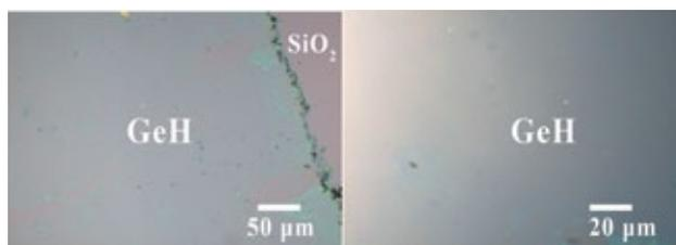
**Figure 4: Optical images of 1.5 nm GeH transfer.** (a) Transferred sample at 10x objective. (b) Transferred sample at 60x objective.
