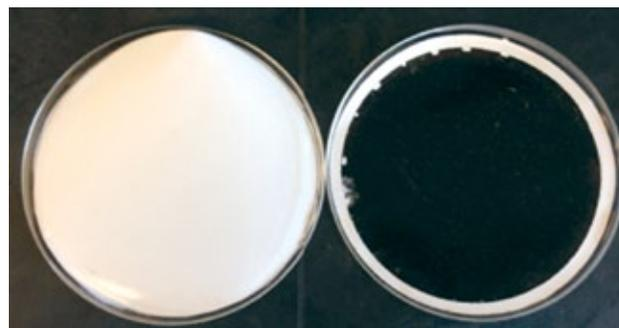
**Figure 1:** PS35 support (left, white) and CNT membrane on a PS35 support (right, black with white ring) (scale bar is 12 cm).
