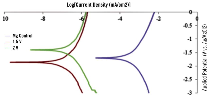
*Figure 2: Potentiodynamic polarization curves of Magnesium anodized in 10 M KOH with subsequent annealing treatment. The scan was performed using simulated body fluid (SBF) at pH 7.4 as the electrolyte. Voltage sweep ranged from -3 V to 0 V at a scanning rate of 100 mV/s.*
