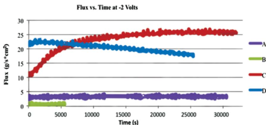
**Figure 8:** Membrane flux during experiment electrical potential difference of -2 volts.
