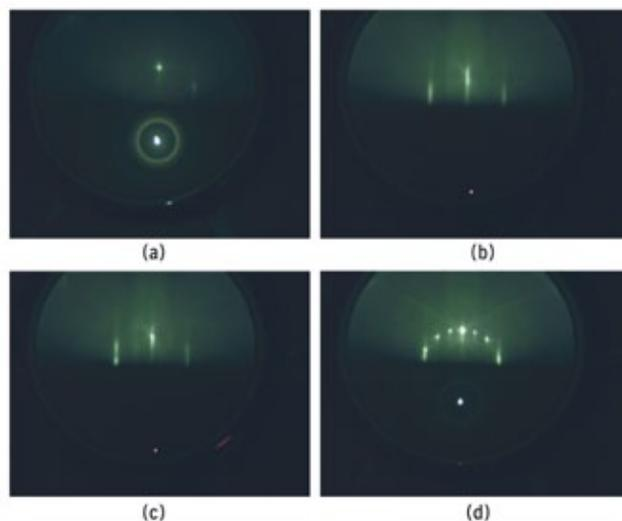
**Figure 2: RHEED patterns of  $\text{CaGe}_2$  growth.** (a) Ge(111) substrate at RT. (b) Ge(111) substrate post-anneal. (c) 5 nm Ge buffer layer. (d)  $\text{CaGe}_2$  growth.
