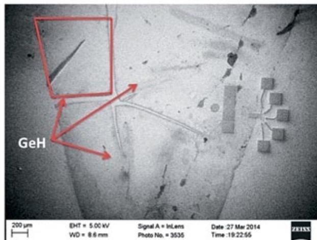
**Figure 5: SEM Micrograph of transferred 1.5 nm GeH layer onto Si/SiO<sub>2</sub> substrate.**
