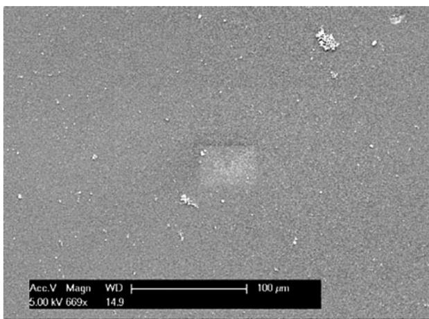
**Figure 2:** Top section view of a SEM image of membrane with PVA and CNTs on a PS35 support (scale bar is 100  $\mu$ m).
