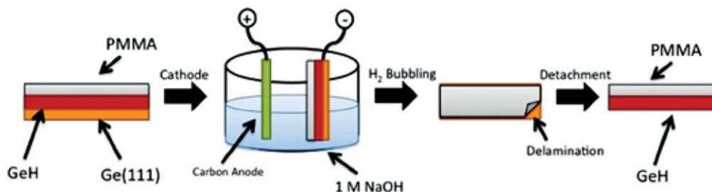
**Figure 3: Electrochemical delamination procedure.** (a) PMMA spin-coat. (b) Cathode and anode placed in electrolysis solution with constant current supply. (c) Hydrogen bubbling occurs between PMMA and substrate. (d) PMMA/GeH layer separated from substrate.
