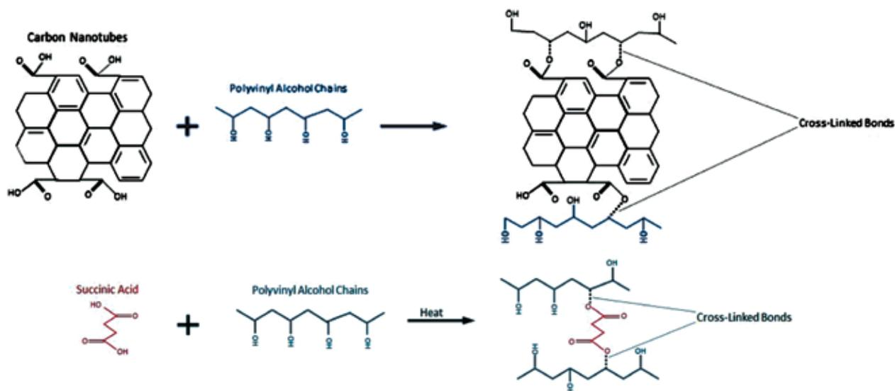
**Figure 5:** Cross-linking of PVA chains, CNT, and succinic acid through reactions with PVA's hydroxyl groups to immobilize CNT within the PVA chain polymer.
